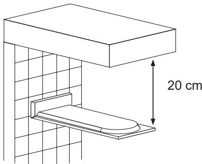
In order to keep you safe and convenient when you install the head shower, the shower should leave the ceiling at least 20 cm, above the above parameters is only for reference.
